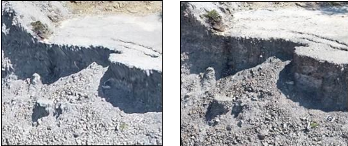
Figure 3: Side by side comparison of the 3D reality model level of detail able to be obtained for near vertical features captured using nadir and oblique capture strategies (left and right images respectively)
