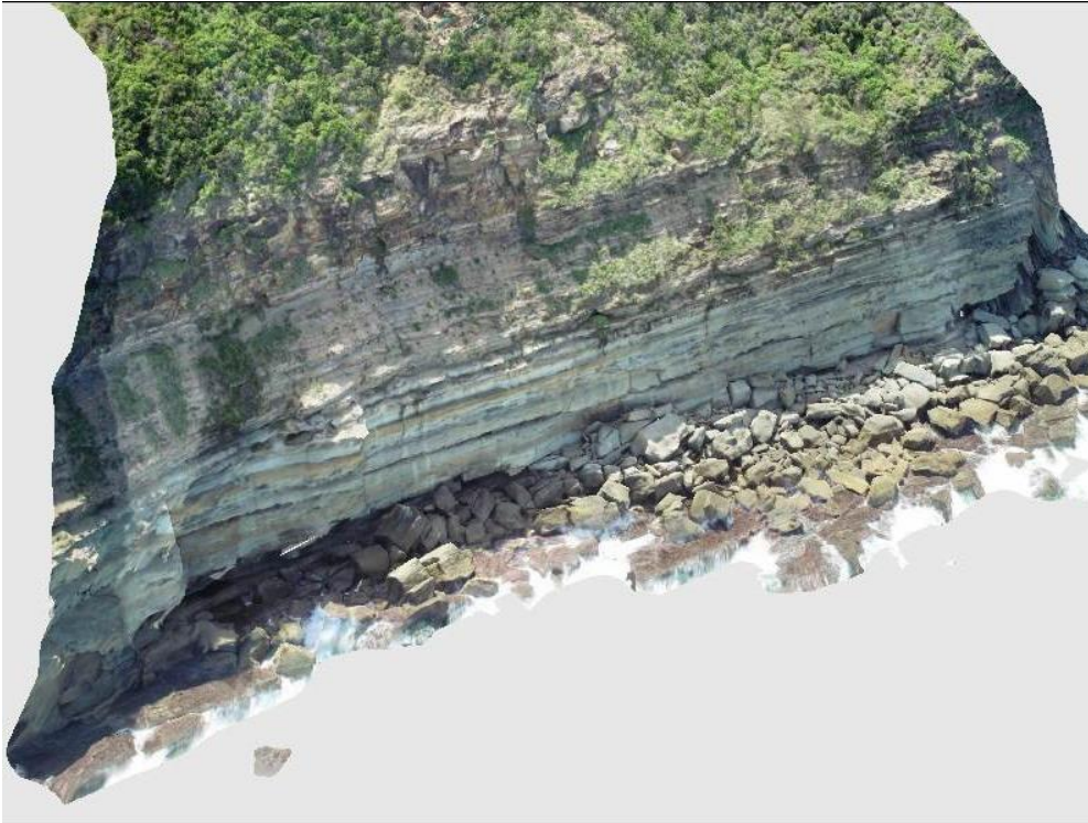
Figure 1: Example of a photogrammetry reality model of 50m high sea cliff
